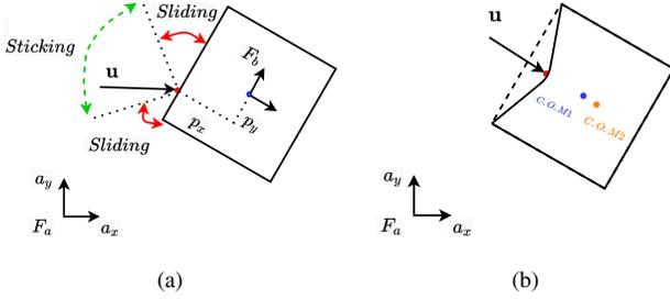
Fig. 2: (a) Kinematics of the rigid slider object in a single point of contact with robot pusher. Dashed green arrow indicates the region for sticking to the contact point, and solid red arrows show sliding zones. (b) Changes in the C.O.M and outer shape of a deformable slider
