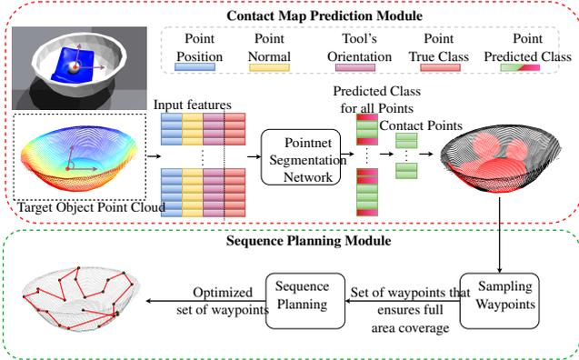
Fig. 2: The proposed planning pipeline consists of: a contact map prediction module learns from target object point clouds, which form the input to a dense point cloud network to produce per-point contacts; a sequence planning module that harnesses the trained prediction model to generate an optimal trajectory to accomplish the task.
