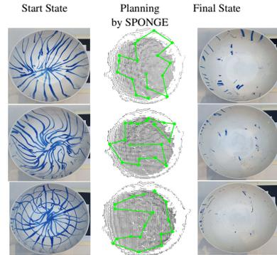
Fig. 5: Qualitative visualizations of *SPONGE* for real-world dish cleaning task. Columns headed by Start State are the target object with blue marker writings denoting dirt need to be removed. The optimal coverage trajectories planned by *SPONGE* (solid green lines) are shown in columns headed by Planning by *SPONGE*. The columns headed by Final State are when robot is done executing the early planned trajectories.
