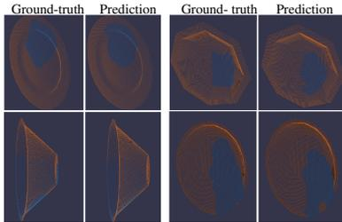
Fig. 4: Visualization of the contact map predictions on the test dataset and the ground-truth in simulation. Left columns show the ground-truth and the right columns show the prediction. Blue indicates points that are in contact with the deformable tool, while orange denotes points that are not in contact with the deformable tool.
