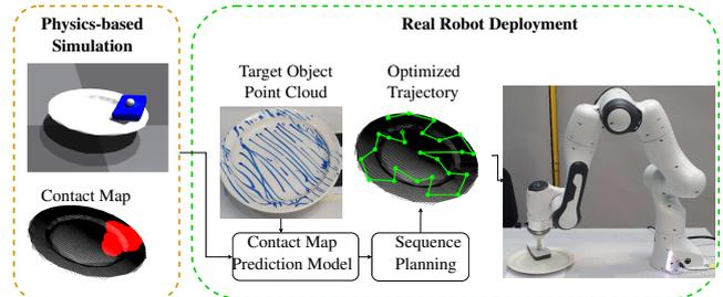
Fig. 1: SPONGE deployed in the real world to accomplish a dish cleaning task with a deformable sponge. Given a point cloud of the target objects, SPONGE powered by a contact map prediction model trained in simulation, plans an optimal trajectory aiming at achieving full area coverage of target objects with the least number of waypoints.
